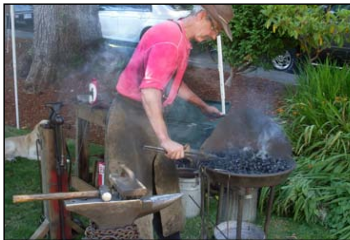
Blacksmith Gary Lewis of the Loan Wolf Forge heats a piece of steel in his forge prior to shaping it on the anvil during Old-Fashioned Fun and Games. Samples of his work can be seen on the web at www.theloan-wolfforge.com .
